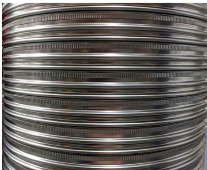
Corrugations of outer skin protect the integrity of the inner skin
